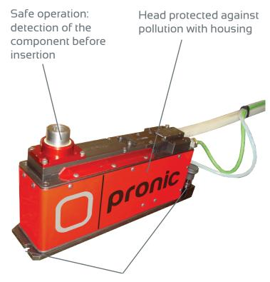
Quick installation kit (no need for special tool) with integrated POKA YOKE mistake-proofing
