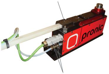
Quick connections for electrical and pneumatic power
