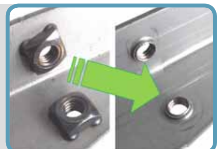
M12 x 1,50 thread • Medium-carbon Steel - Thickness: 3 mm • Thread depth: 19 mm Pull test: >95 000 N
