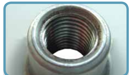
M12 x 1,50 thread • Medium-carbon Steel - Thickness: 3 mm • Thread depth: 19 mm Pull test: >95 000 N
