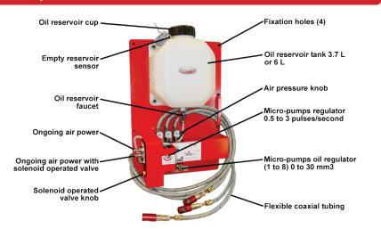
The micro-pumps push the oil into the micro-lubrication nozzles then an air flux sprays micro-droplet directly on the working zone of the tap. Depending on the hardness of the material to be tapped, the oil volume and number of pulses per cycle can be adjusted. The oil consumption is so low that it is not necessary to plan on recycling the lubricant.
